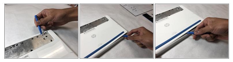
• Starting in the top right-hand corner of the exposed metal piece, use the blue plastic opening tool to remove the back panel.
