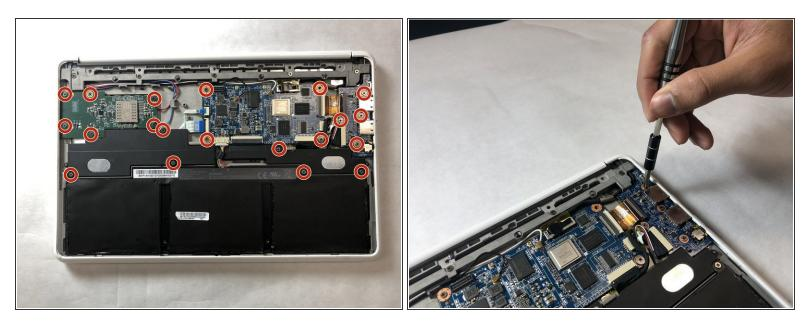
• Remove twenty 3.42mm screws with the Phillips #1 screwdriver.
