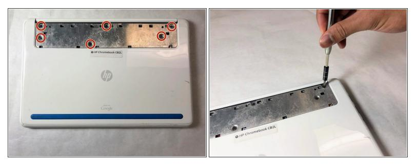
Remove six 4.77mm screws using the Phillips #1 screwdriver.
