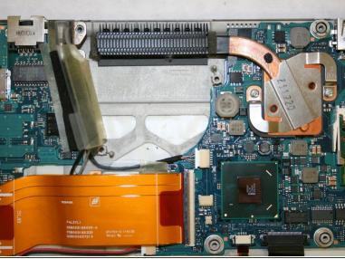
The fan is now free and able to be removed. Lift the fan out of place.
