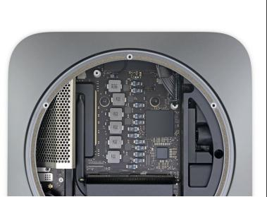
Use a T10 Torx driver to remove the two 7.5 mm screws securing the logic board.
