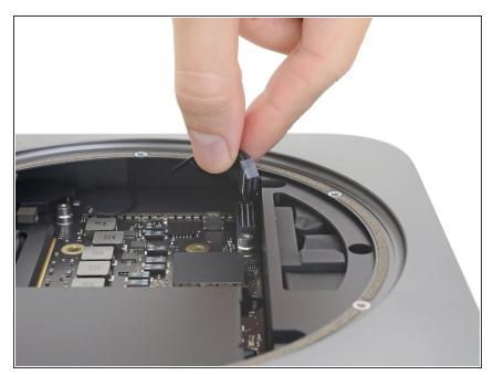
Grasp the power supply cable and lift to disconnect it from the logic board, wiggling as needed to loosen it up.
