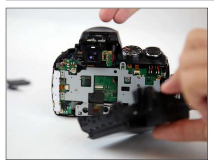
Now that the ribbon cable is unconnected, pull away the frame to work on.
