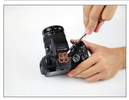
With the Phillips #00 screwdriver, remove all four screws.
