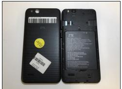
Remove back cover of the device from the crease of the bottom left corner using opening tool or fingernail.
