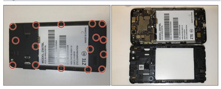
• Unscrew all 16 screws from the mid-frame with a J000 screwdriver.
