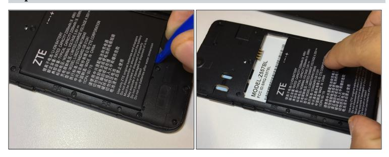
• Remove the battery with an opening tool or fingernail.
