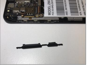
Carefully use a pair of bent nose tweezers to pull out the button cover. I should come
