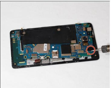
Desolder and remove in front of the motherboard.
