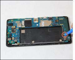
Unplug wires by pushing up with the plastic opening tool
