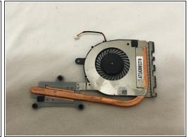
Remove the heatsink and fan from the motherboard. You can now clean or replace it as you see fit.
