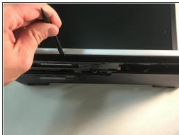
Carefully pry off & loosen the bottom base.
