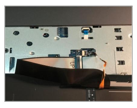
Unplug the keyboard cable & remove the keyboard.
