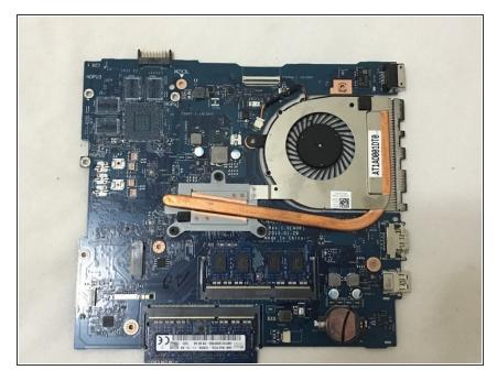
After removing the bottom base, you can access the heatsink and fan, which is attached to the motherboard.
