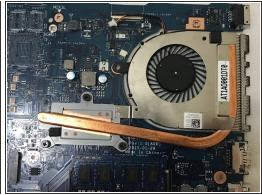
Unplug the cable that connects the heatsink and fan to the motherboard.
