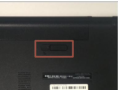
Flip the laptop with the serial number facing up. You should be able to see the battery release switch.
