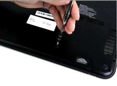
Using the Phillips #0 screwdriver, remove the two 7 mm screws from the back casing.
