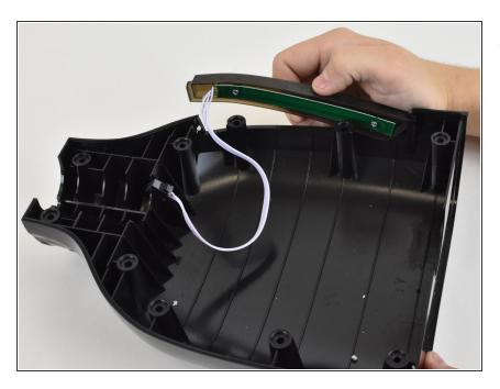
Grab the wire of the connector you disconnected from the case earlier and slide the entire light out away from the case.
