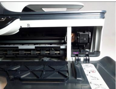
• Insert 2 fingers in the dent on the right side of the printer and pull towards the front of the printer.
