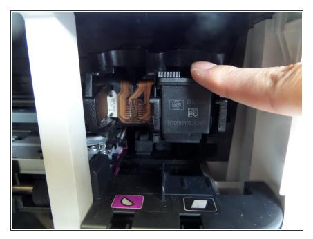
Use a finger to push down on the top of cartridge.
