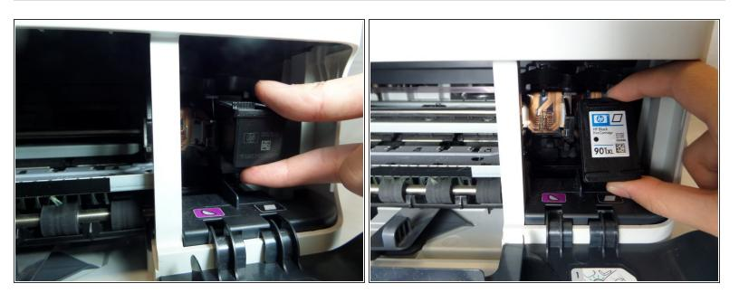
Pull the cartridge out towards the front of the printer.
