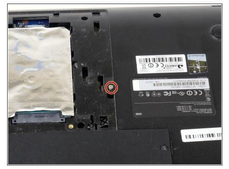
Find the screw between the hard drive and the model label. Then remove the M2.5X5 screw with a Phillips #0 screwdriver.
