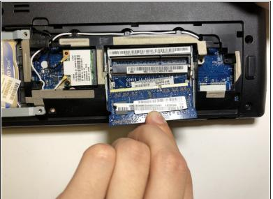
Use two plastic opening tools to pry the two clips outward to release the RAM chip.
