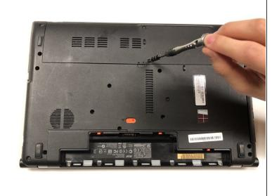
Remove the two 5.3 mm Phillips #0 screws.
