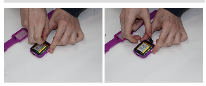
• Carefully remove the speaker from the case without disconnecting it from the motherboard.
