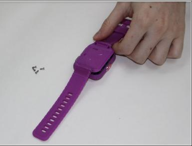
Next, use the Phillips #00 screwdriver to unscrew the four 6.0 mm screws located in each corner of the watch to remove the backplate.
