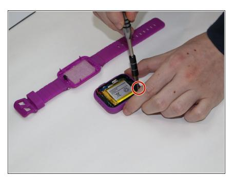
Using a Phillips #00 screwdriver, remove the 0.6 mm screw.
