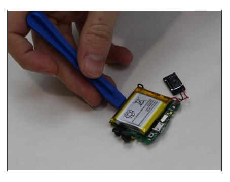
Carefully pry the battery off of the circuit board using the plastic opening tool.
