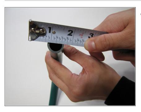
Measure the diameter of the inside of the original hose.
