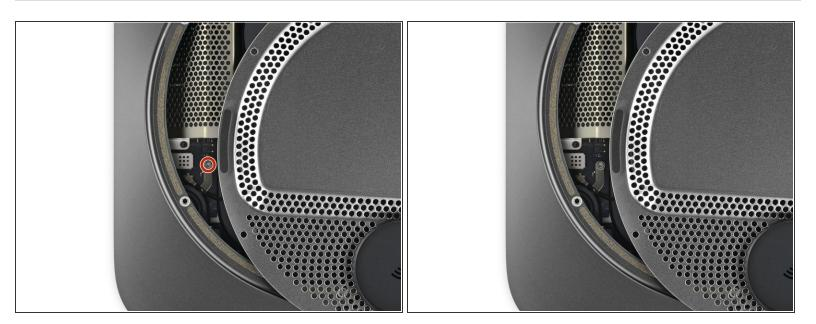
Use a T6 Torx driver to remove the 2.8 mm screw securing the antenna cable to the Mac mini's logic board.
