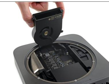
↑ Don't try to remove the fan completely in this step—just lift it so you can access the cable underneath.
