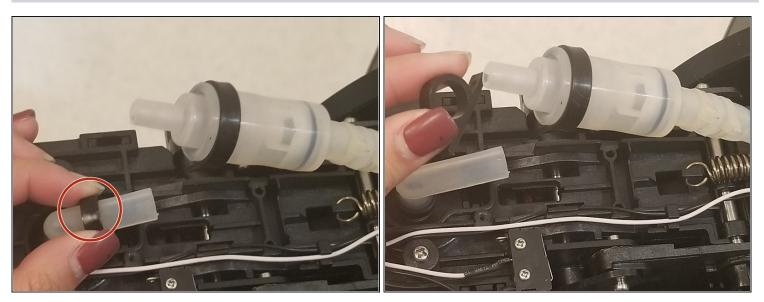
• Slide the black plastic ring, which holds the puncture needle tube down, off of the tube.
