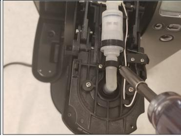
• Using a Phillips #0 screwdriver, remove the two 7.0 mm screws located on the sides of the tube near the puncture needle.
