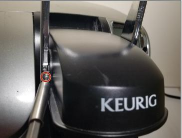
• Using a T15 Torx screwdriver, remove the two 29.0 mm screws on each ends of the handle.
