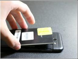
Pull up on the small indention on the right side edge and remove the back portion of the phone.
