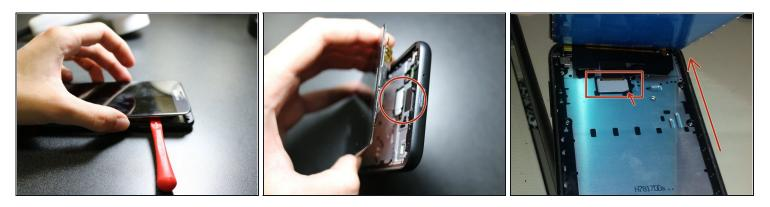
• Gently lift lower side and loosen all edges to hinge screen up from bottom.
