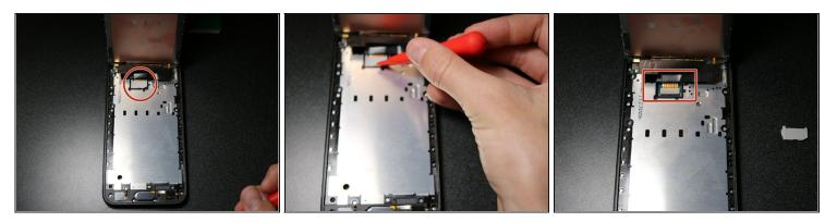
• Use your prying tool to slowly pry up on the **bottom right corner** of the white cable guard, exposing a thin ribbon cable connector.
