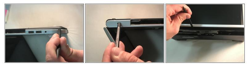
• Carefully pry off & loosen the bottom base.
