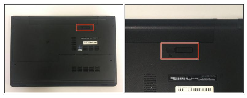
Flip the laptop with the serial number facing up. You should be able to see the battery release switch.
