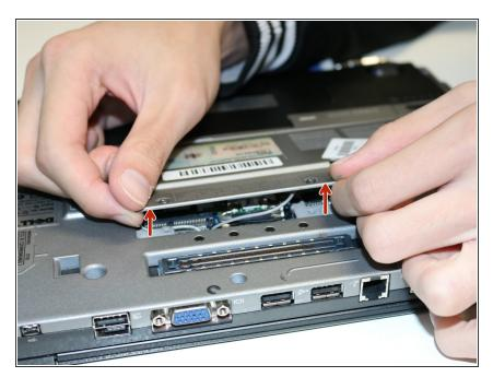
Once all 3 screws have been removed, carefully remove the panel by grabbing the edges, and pulling up.
