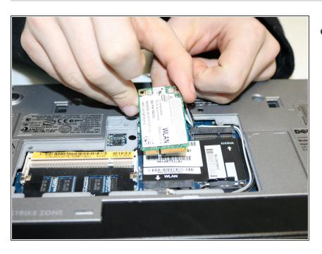
Pull the wireless adapter out away from where it was connected.
