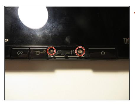
After removing the buttons, remove the two screws marked.
