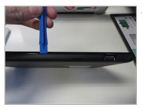
Carefully pry off the outer perimeter of the tablet using a plastic opening tool.
