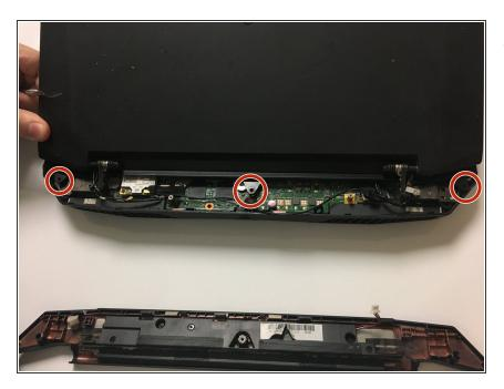
Turn the laptop over and remove the screws as shown
