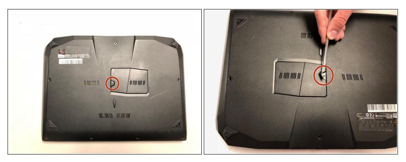
Lift the screw cover and remove the screw using a Phillips #0 screwdriver.
