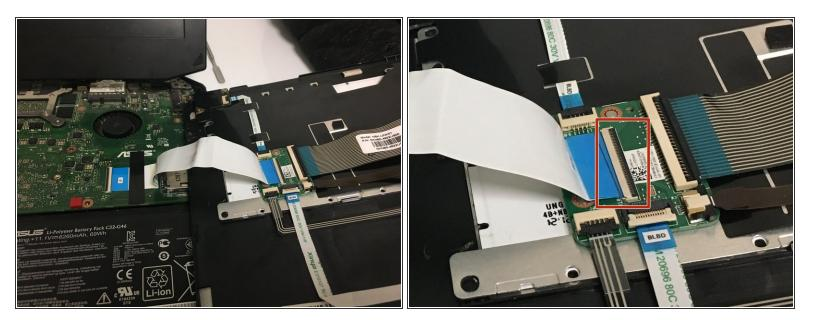
Detach the ribbon cable by releasing the clip
