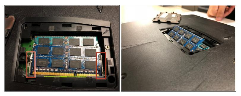
• Push outwards on the clips to release the RAM stick. The stick should pop up at an angle.
