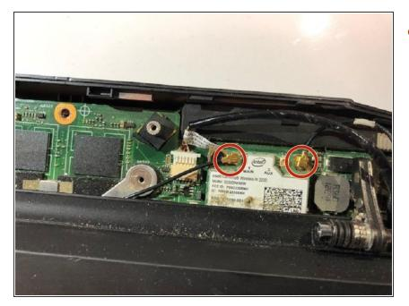
Remove tape and gently pull up on golden cap connectors to disconnect them.
