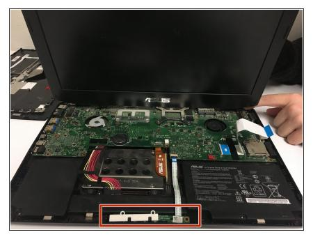
With the motherboard exposed, locate the Indicator Lights and their white plastic housing piece.
