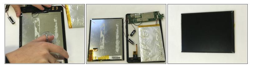
• Use the suction cup to loosen and pull up the screen.
