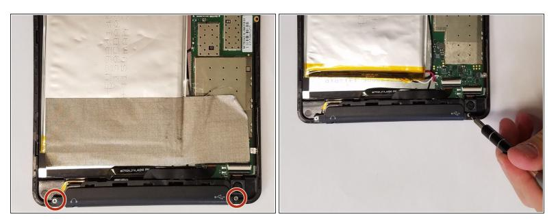
• Using a JIS #000 screwdriver, remove the two 2.5 mm screws.
