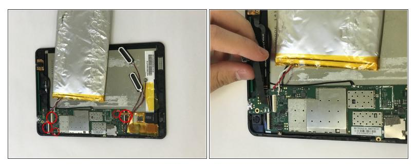
Remove all wire connections by sliding them out of the connectors.
