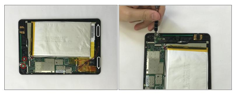
Remove the two JIS #000 screws.
