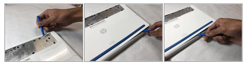
• Starting at either the top left or right hand corner of the exposed metal piece, use the blue plastic opening tool to remove the back panel.
