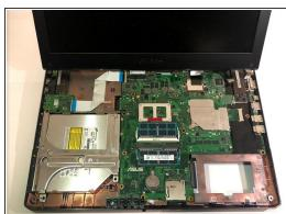
Remove the ribbon connectors that connect the keyboard to the motherboard. The keyboard should now be completely disconnected from the laptop.
