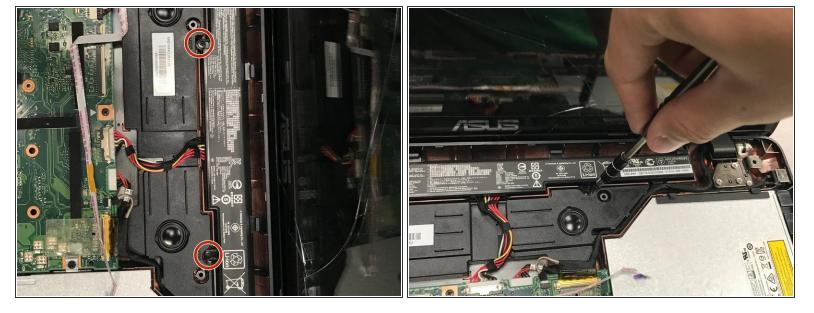
Remove the two 7mm screws holding the battery in place using a Phillips #00 screwdriver.
