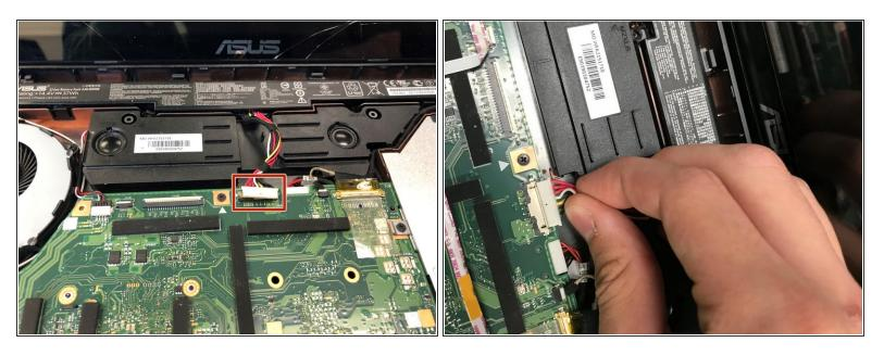
• The battery contains wires connecting it to a circuit board. Slowly pull up and disconnect the wires from the board by pulling on the white tab.
