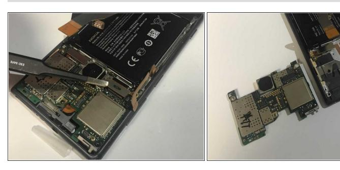
Remove the motherboard by sliding tweezers between it and the back of the screen. Lift up.
