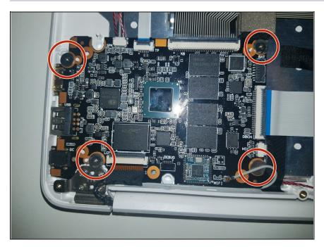
Remove the screws located in the corners of the board using a J00 screwdriver.
