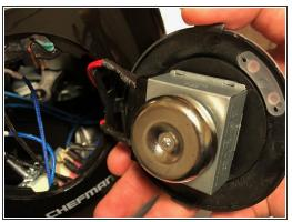
Squeeze on plastic pieces holding timer down and push out.
