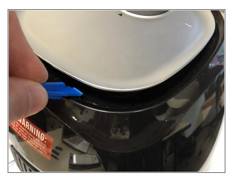
Using the plastic opening tool, pop off each of the four corners on the top silver plate.
