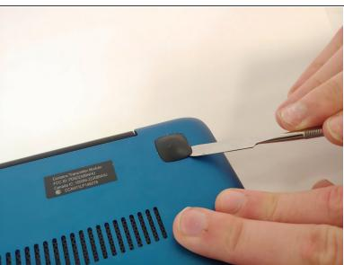
Using the metal spudger, remove all the rubber squares on the bottom of the laptop.
