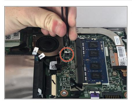
Disconnect fan cable with tweezers.
