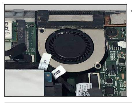
Remove the processor fan and heat sink assembly.
