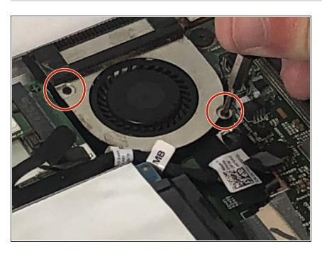
Use a screwdriver to remove the two 2.3mm PH00 screws on the processor fan.
