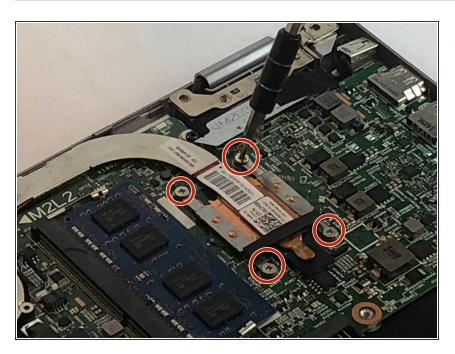
Use a PH0 screwdriver to loosen the 4 captured screws on the heat sink assembly.
