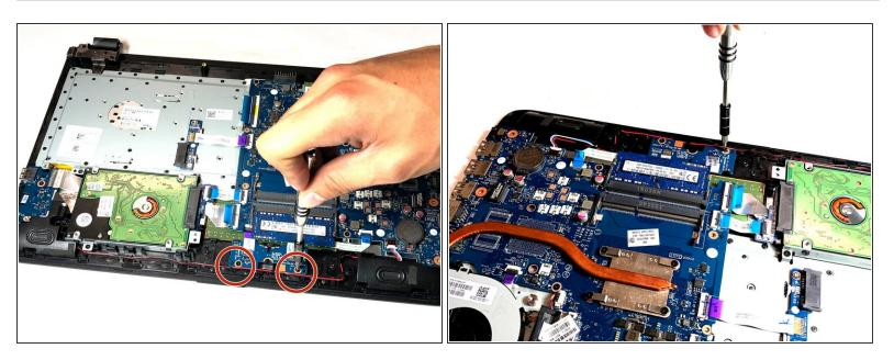
Remove the two 3.3mm Phillips-head screws that secure the trackpad circuit board to the top cover.
