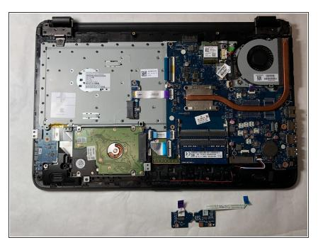
• Lift and remove the trackpad button circuit board.
