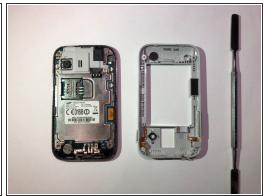
• Use the metal pry tool to separate the interior back panel from the interior hardware and screen.
