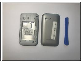
• Use the blue plastic opening tool to pry the back-panel off of the device.
