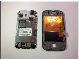
Disconnect the orange motherboard connection, then remove the interior hardware from the front screen display.
