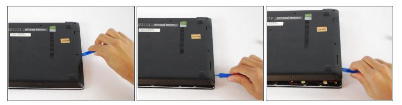
• Use a plastic opening tool to gently pry the bottom of the laptop up. Slowly slide it along the edges, twisting it every so often to pop the bottom of the laptop out of the clips holding it in place.
