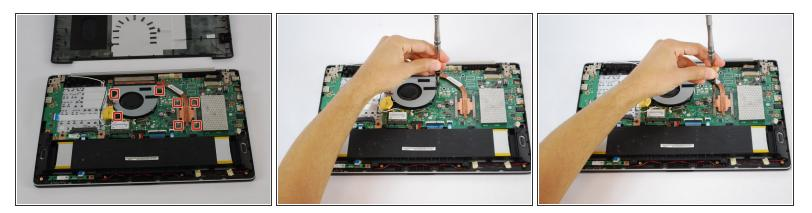
Using a Phillips #1 Screwdriver remove the three 3 mm black screws and four 2 mm copper screws holding the fan and heat sink in place.
