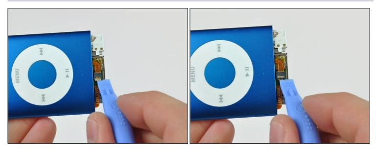
• Use the edge of an iPod opening tool to flip the ZIF cable lock up toward the headphone jack.
