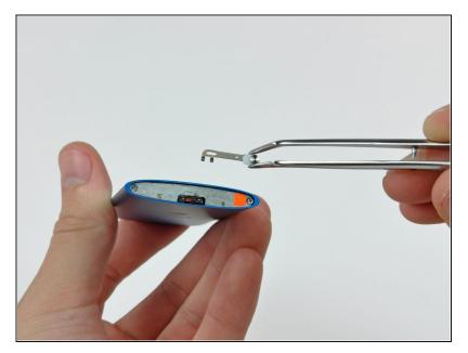
• Remove the hold switch slider from the top of the Nano.
