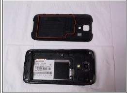
• Use the tab marked "PULL" to remove the battery from its enclosure.
