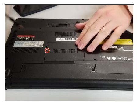
Use a Phillips #00 screwdriver to unscrew the single RAM cover screw.
