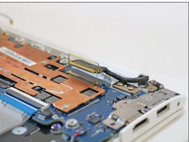
Lift hinge on connector up and pull the connector away from the device.
