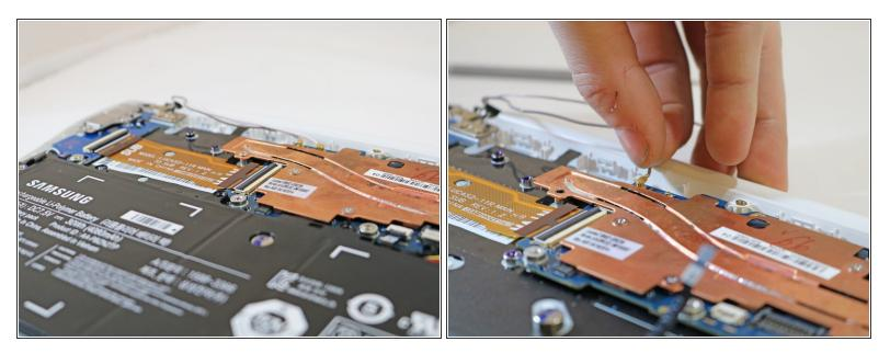
Remove auxiliary wires for microphone and webcam.
