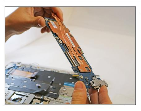
Remove the motherboard from the device.
