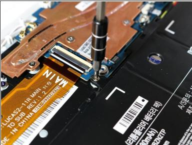
Remove four, 5mm Phillips #0 screws connecting the battery to the laptop
