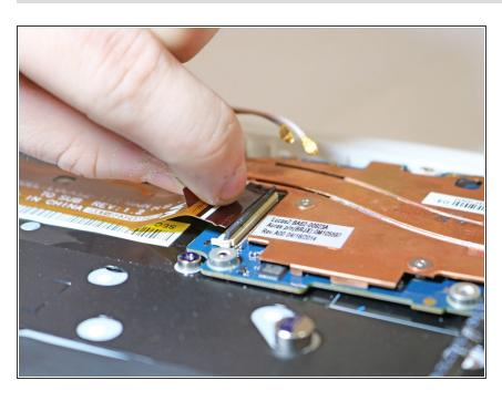
Remove the connector for the motherboard and sub-board.
