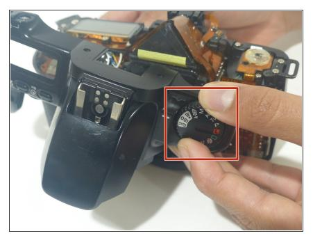
Locate the camera dial (surrounded by a red square) and turn the top cover of the camera upside down for access to the screw underneath the dial.
