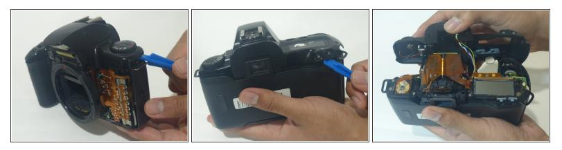
• Using an opening tool (you can also use your nails, but try not to use something potentially damaging to the camera such as metal), separate the top cover from the rest of the camera!
