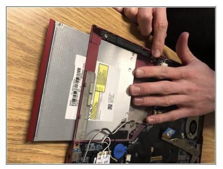
Once you have unscrewed all the screws, push in and slide out the disk drive from the device.
