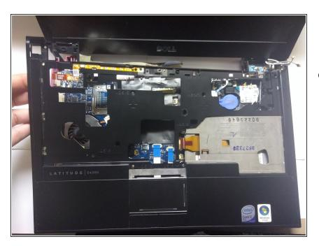
Lift the keyboard panel to separate the component from the rest of the device.
