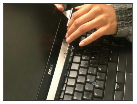
Open the laptop and remove the small panel located above the keyboard.
