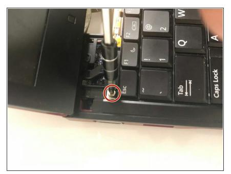
Using a Phillips 1 Screwdriver, unscrew the three M2x3-mm screws located above the keyboard where the small panel was originally.
