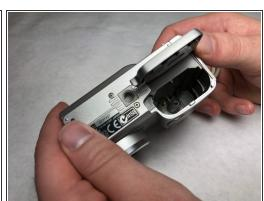
• Flip up the cover and remove the battery inside the slot.
