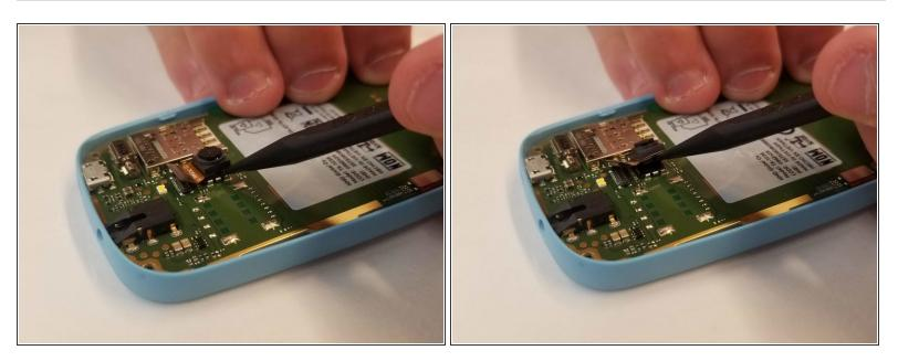
• The camera is held in with double sided and foam. Using the spudger, lift up on the camera to remove it from the motherboard of the phone.
