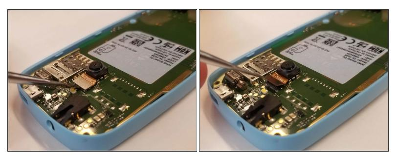
Using the pointed metal spudger from the metal spudger set, insert the tool underneath the small snap clip, and disconnect it by lifting it up.
