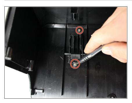
Inside the panel, remove the two 6mm #1 Phillips head screws.
