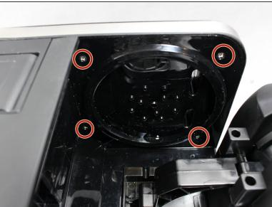
• Remove single 6mm #1 Phillips head screw from the side of the unit and four 6mm screws from under the basket area.
