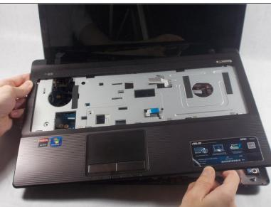
Separate the front plate of the laptop from the back using the plastic opening tool.
