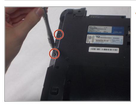
Remove the two 2mm screws using a Phillips #1 screwdriver.
