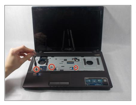
Flip the laptop over again, open it, and unscrew the three 7mm screws using a Phillips #1 screwdriver.
