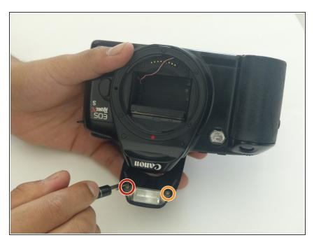
Using a <u>PH000 screwdriver</u> bit, remove the two silver screws circled in the picture. Both screws are 5 mm in length and about 1.25 mm in diameter. To reassemble your device, follow these instructions in reverse order.
