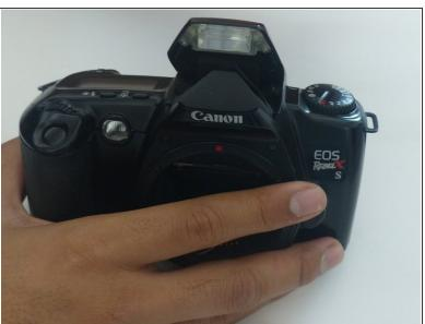
• Pull up on the flash / the camera part housing the flash, as shown in the pictures. If this isn't working, try these things not shown in the pictures: 1) using a spudger, your nail, or the like to pry it open; or 2) pull it open with your finger and thumb on either side of it.
