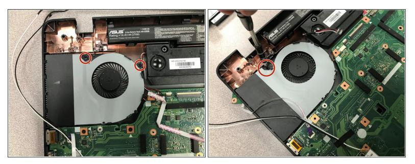
Remove the two screws directly above the fan.
