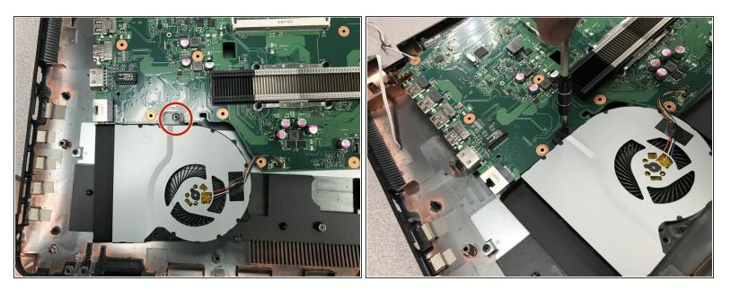
Remove the Phillips #00 screw that holds the fan to the motherboard.
