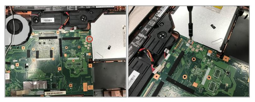
• Remove the one screw on the right side of the motherboard that keeps the cd tray in place.
