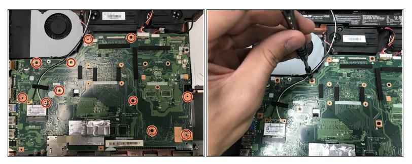
Unscrew the 11 screws that hold the motherboard to the base of the computer with a 00 Phillips screwdriver.
