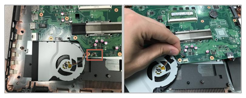
On the bottom of the motherboard, locate the wire plugged in and pull it out to completely detach the fan from the motherboard.
