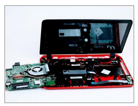
Detach by lifting the motherboard up and flip the motherboard over.
