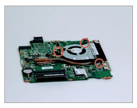
Remove all three screws that hold the fan to the system board
