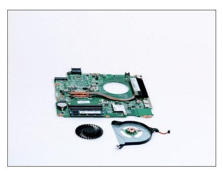
Lift and remove the fan from the top cover.
