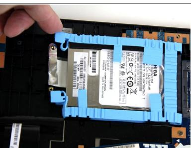
The hard drive is held in place with a soft, blue rubber retainer. The retainer can be disconnected
