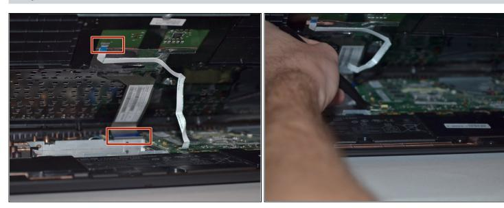
• Lift palm rest and unplug keyboard cable and touchpad cable using tweezers. After these two cables have been unplugged you can remove the keyboard cover panel.
